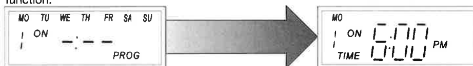
FIG 5: Setting the timer to turn on at 6 PM each Monday for Program 1
