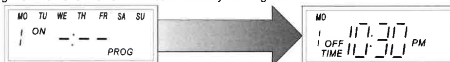
FIG 6: Setting the timer to turn off at 10:30 PM each Monday for Program 1
