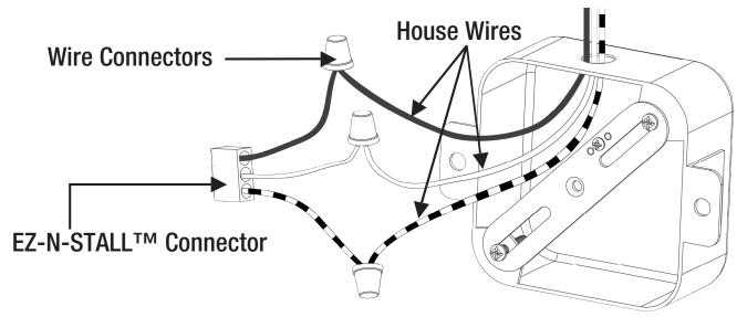
• Push EZ-N-STALL™ Connector into EZ-N-STALL™ Clip and place onto mounting bar.
