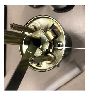
Insert the fork end of the pickle tool down the spring housing with the flat of the tool aligned with the screw posts.
