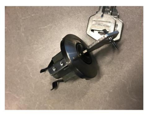
Test the key by rotating in both directions. To remove the key, turn to vertical position and pull it out. Make sure the C clip is securely in position before doing this.
