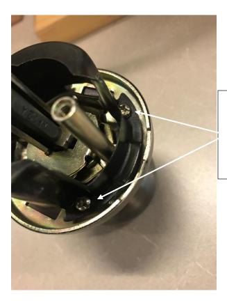
For the final step, Re-attach the metal body with the two screws
