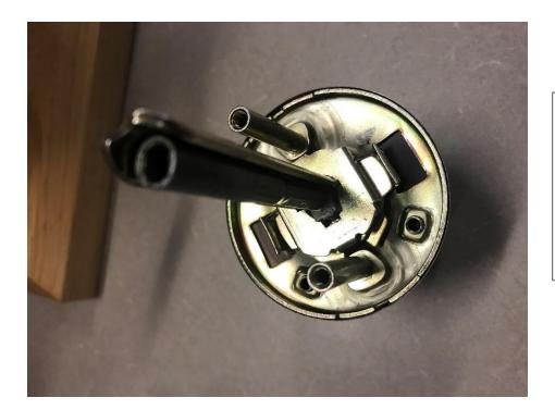
Slide the locking spindle into the spring housing until you hear it click into place.
