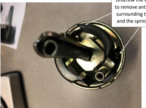
Unscrew the two screws to remove anti-pry shield surrounding the spindle and the spring housing.
