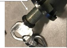
It is important to use the Plug Follower so the top pins and springs do not fall from the cylinder
