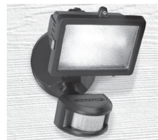
Position floodlight to illuminate desired area, but allowing a minimum of 2 inches away from fixture housing, and so that the bulb is horizontal (within 2 degrees). Aim the motion sensor at the center of the desired detection area.
