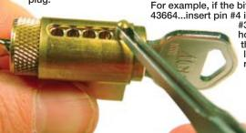
43664...insert pin #4 into the first hole, pin #3 into the second hole, and pin #6 into the third hole, and likewise for the remaining chambers.
