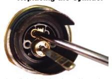
Replace the cylinder in the housing and insert the retaining
