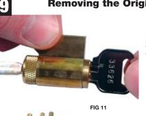
Dump the pins out. It may be helpful to move the kev slightly back and forth to help eject the pins (FIG 11).
