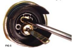
Remove the screw using a Phillips head screwdriver and set the screw aside.
