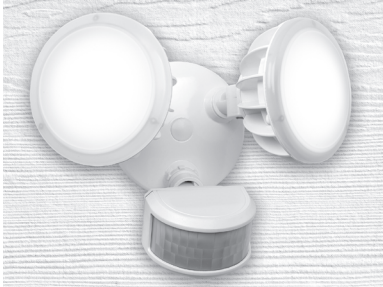
Position lamp holders downward at a minimum 45° and away from fixture housing a minimum of 2 inches. Aim the motion sensor at the center of the desired detection area.
