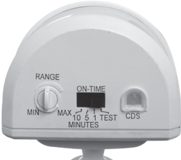
Observe the two controls on the bottom of the sensor. The RANGE (sensor sensitivity) control is located on the bottom left. The ON-TIME (duration) switch is located on the bottom center.
