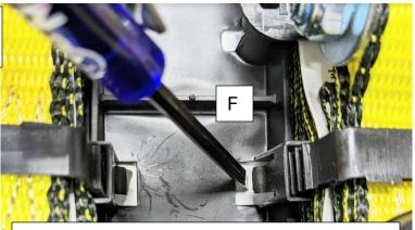
Push your screwdriver through this hole and the paper on the back as shown in (F).
