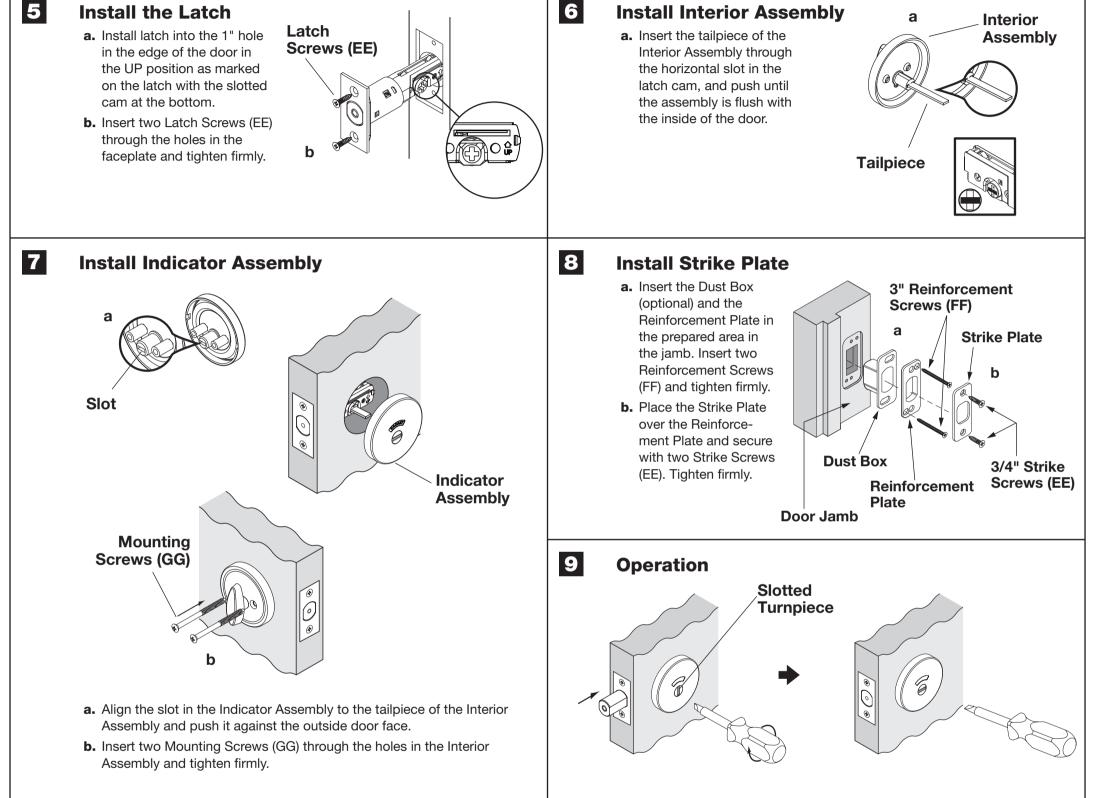
For an emergency situation, the slotted turnpiece in the Indicator Assembly can be rotated using a flathead screwdriver to retract the bolt.
